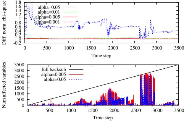
Fig. 5: How the backsubstitution threshold  $\alpha$  affects accuracy (top) and computational cost (bottom) for the Manhattan dataset. For readability of the top figure, the normalized  $\chi^2$  value of the least-squares solution was subtracted. A small threshold such as 0.005 yields a significant increase in speed, while the accuracy is nearly unaffected.
