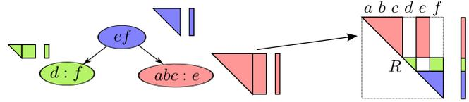
**Fig. 3:** Connection between Bayes tree (left) and square root information factor (right): Each clique of the tree contains the conditional probability densities of its frontal variables. In square root information form these are the same entries as in the corresponding matrix factor  $R$ .
