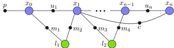
Fig. 2: Factor graph [25] formulation of the SLAM problem, where variable nodes are shown as large circles, and factor nodes (measurements) with small solid circles. This example illustrates both a loop closing constraint  $c$  and landmark measurements  $m$ , in addition to odometry measurements  $u$  and a prior  $p$ . Note that arbitrary cost functions can be represented, also including more than two factors.
