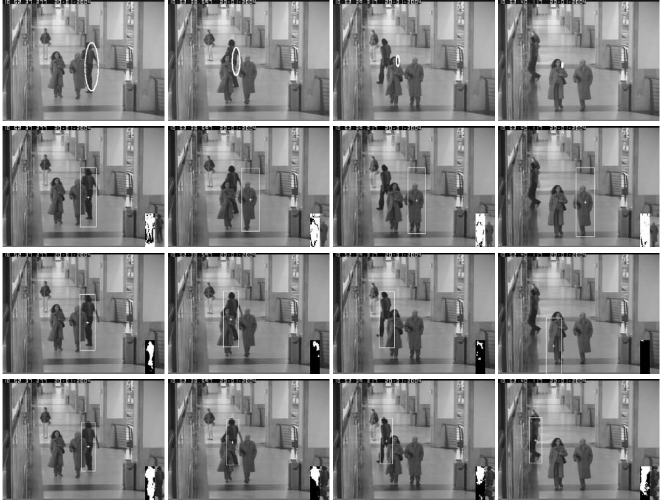
Figure 5: Comparison of different algorithms in handling a challenging long-term occlusion. The four rows from top display the results of the algorithms of [4], [7], [12], and our proposed algorithm, respectively. The four columns from left show frames 1980, 2013, 2032, and 2052, respectively. In the first row, the tracking result is represented by an ellipse. In the remaining rows, the tracking result is indicated by a rectangle with a cross at the center. For rows 2 and 4, the current occlusion situation of the target (or template mask) and the current template are displayed from left in the lower right corner of each image. For row 3, only the current occlusion situation of the target is displayed in the corresponding positions. Occluded pixels are indicated in black.
