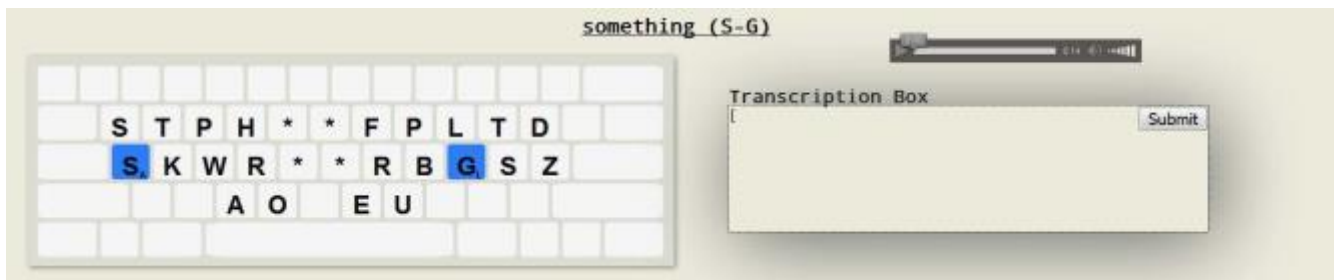
Figure 3. The user interface for Scopist highlights stenotype keys on a typical qwerty layout to teach a crowdworker the appropriate hand posture for chording. The highlighted keys are for the prompted word underlined at the top of the page, and a reminder of the link between the chord keys and the sounds of the prompted word are provided in parentheses.
