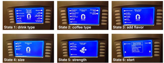
Figure 12. VizLens::State Detection detects screen state and adapts to it. In this example, VizLens figures out which of six states this fancy coffee machine is in, and provides feedback or guidance specific to that screen.
