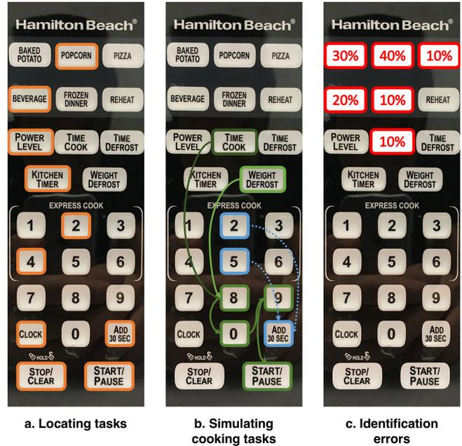
Figure 7. Visualization of user study tasks and identification results. (a) Locating tasks highlighted in orange. (b) Simulating cooking tasks highlighted in green and blue, and sequences shown with line and dashed arrows. (c) Identification errors visualized on the interface, where all errors are happening on the top region of the control panel.
