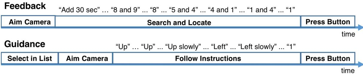
Figure 9. Time breakdown for feedback and guidance modes. For feedback, users aim the camera and search for the button repetitively, and press once they reach the button. For guidance, users first select a button in the list, aim the camera, then follow the instructions to the button, and press.
