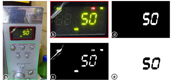
Figure 13. VizLens::LCD Display Reader applies OCR to recognize digits on the portion of the interface that is an LCD screen. (a) Separated dynamic and static regions. (b) Image sharpening using unsharp masking. (c) Intensity-based thresholding. (d) Morphological filtering and small blob elimination. (e) Selective color inversion.
