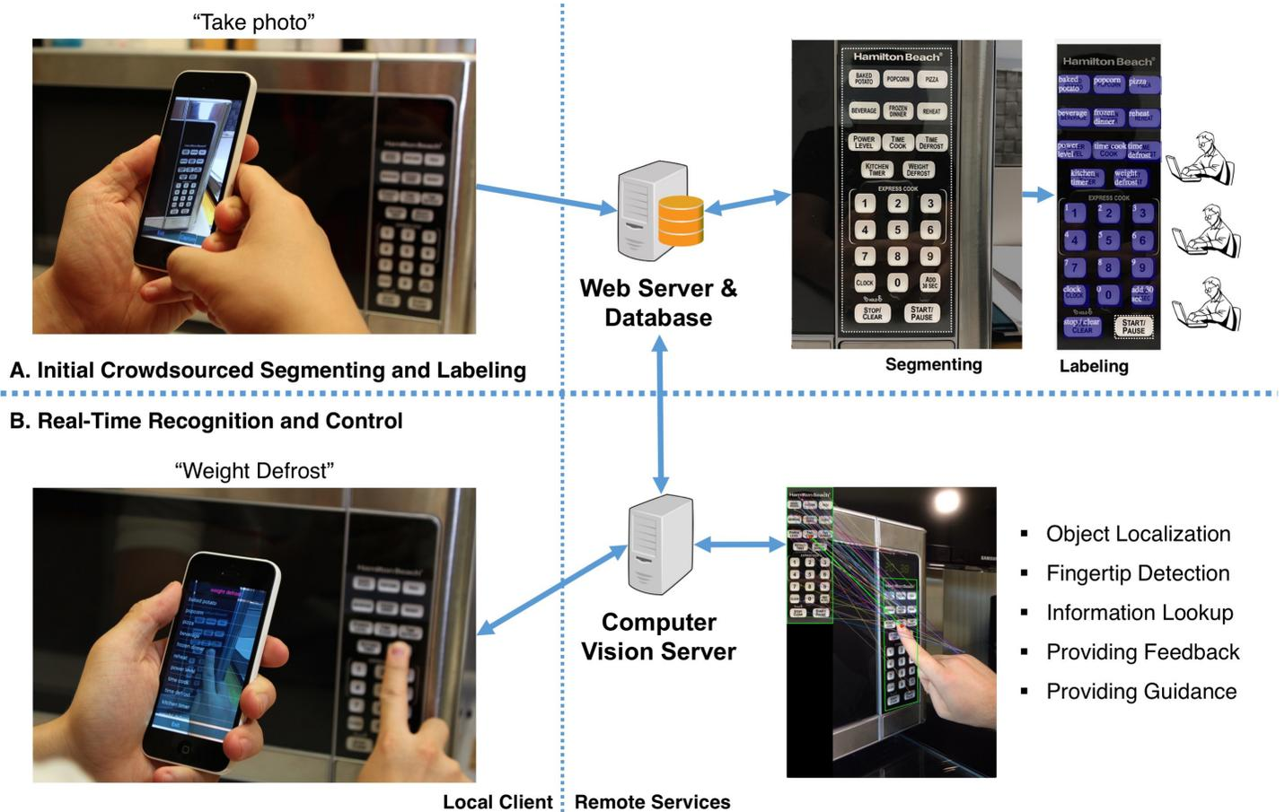
**Figure 1.** VizLens users take a picture of an interface they would like to use, it is interpreted quickly and robustly by multiple crowd workers in parallel, and then computer vision is able to give interactive feedback and guidance to users to help them use the interface.
