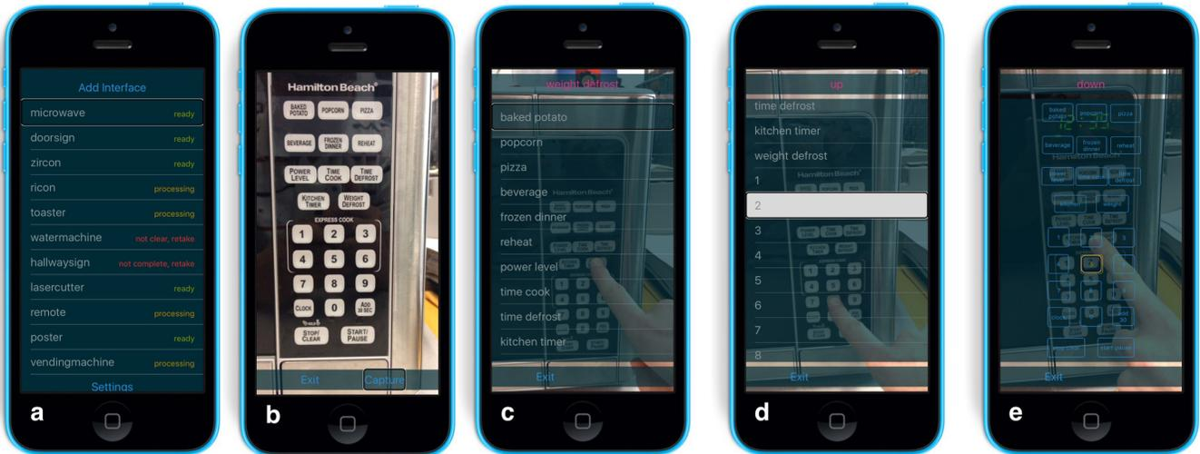
**Figure 2.** VizLens mobile app interfaces. (a) App’s main screen, listing all available interfaces and status, as well as Add Interface and Settings options. (b) Interface for Add Interface, where the user can take a photo and denote a name for it. (c) When user selects an interface, he can start to get feedback. (d) When selecting a visual element, the app start providing guidance. (e) a virtual interface layout that users can explore directly on the touchscreen.
