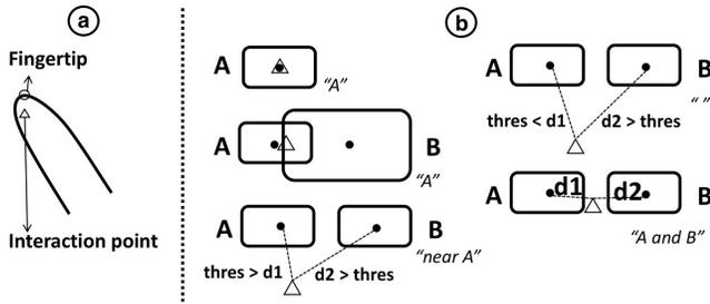
**Figure 5.** (a) Defining interaction point relative to the detected fingertip location. (b) Rules for assigning feedback based on button layout.
