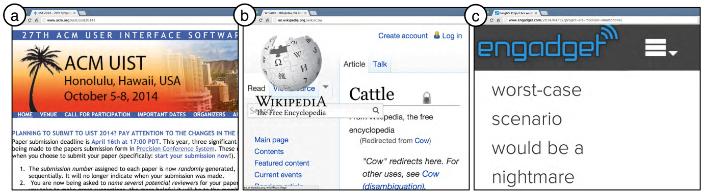
Figure 2. Illustrated examples of three of the most common problems introduced by web magnification: (a) graphical zoom introduces horizontal scrolling, (b) responsive design works well to adapt a web page to higher levels of magnification but often results in overlapping content as magnification grows too large, and (c) as the size of text grows too large relative to its container the lines of text become undesirably thin.
