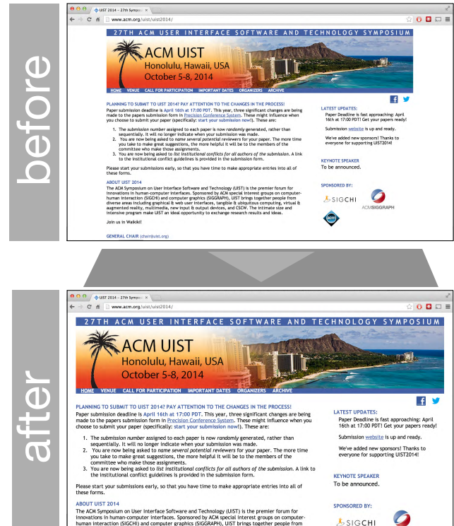
Figure 5. The observed result of applying oppaccess.js to the UIST 2014 web page. In the after screenshot the page is automatically magnified to 1.3x the original, while ensuring that negative effects (horizontal scrolling, overlapping elements, or narrow word-wrapping) are not introduced. This may seem like a small change, but can improve the realized accessibility of this web page for many people with low vision.
