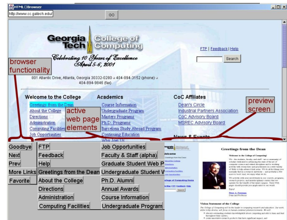
Figure 1: A web browser modified to work with four switch neural-signal users
