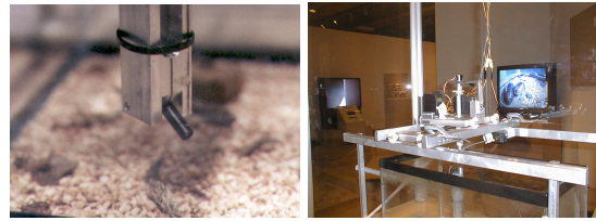
Figure 5: The Toshiba micro-camera remote head and the robot raster
