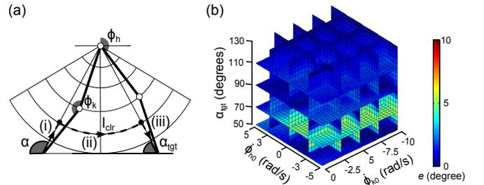
Fig. 2. Robust swing leg controller. (a) The swing controller reaches  $\alpha_{tgt}$  while ensuring ground clearance  $l_{clr}$ , and uses hip ( $\phi_h$ ) and knee ( $\phi_k$ ) angular data as sensory inputs. The knee controller follows a three-part control sequence (details in text). (b) The placement error  $e = |\alpha_{tgt} - \alpha_{td}|$  is shown for largely different initial angular velocities ( $\alpha_{td}$  is leg angle at touch down).
