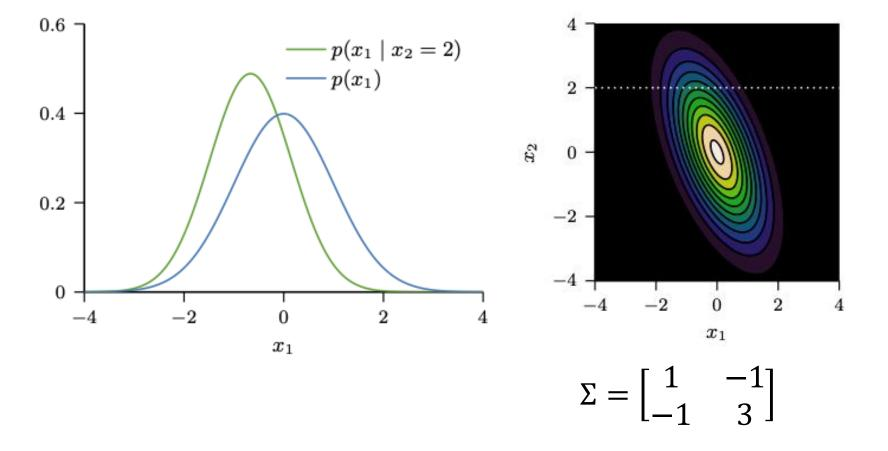
Condition distribution of  $x_1$  given  $x_2 = 2$  for the shown 2-dimensional Gaussian
