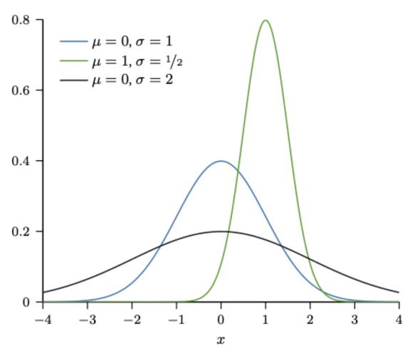
Examples of Gaussian probability density functions for the shown parameter value pairs
