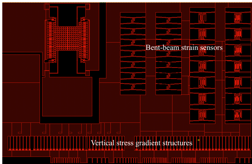
Figure 14: Layout of bent-beam strain sensors for determination of residual stress and various length beams for vertical stress gradient measurement.
