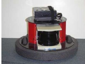
Figure 1. The Botrics Obot mobile robot, equipped with a SICK scanning laser range-finder, which has a  $180^\circ$  sensor field.
