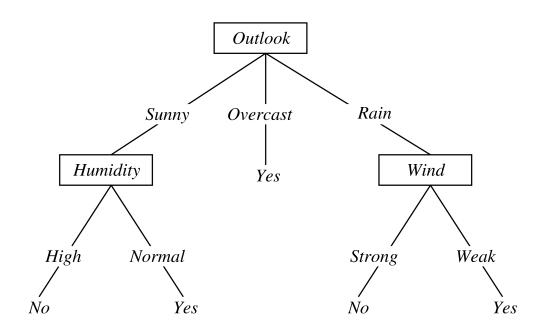
Each internal node: test one feature X<sub>i</sub>
