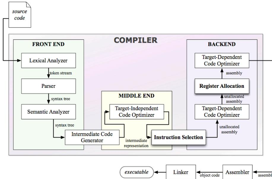
Figure 1: Structure of a typical compiler<sup>2</sup>
