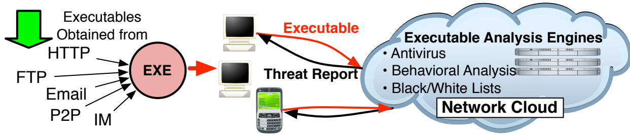
Figure 1: Architectural approach for in-cloud executable analysis.
