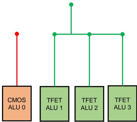
In dispatch stage, identify the producer-consumer pairs in small window, and steer the producer to CMOS ALU.
