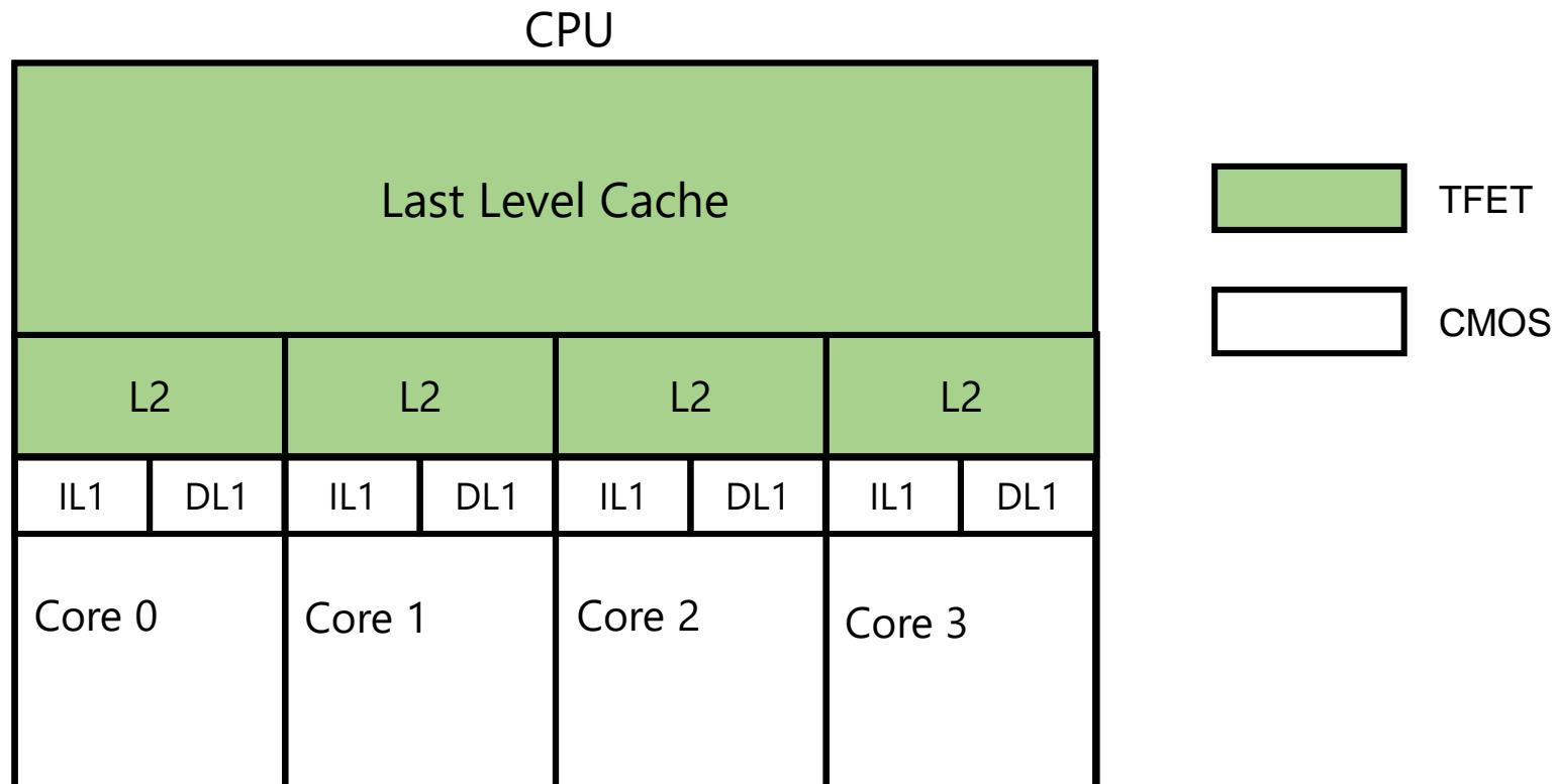
L2 and LLC primarily consume leakage power → TFETs can reduce leakage power substantially
