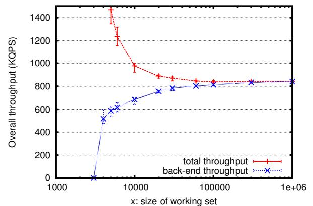
**Figure 10: Throughput that the adversary can obtain by querying for different numbers of keys when the cluster has 85 back-end nodes and  $c = 3000$ . Results for  $x < 3000$  are omitted because all queries would be served by the front-end cache.**
