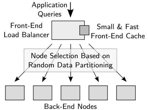
Figure 1: Small, fast cache at the front-end load balancer.
