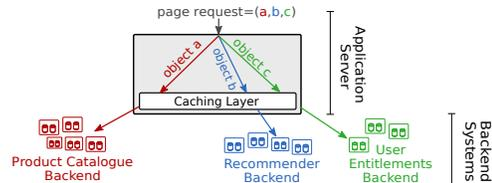
Figure 1: In large webservices, application servers assemble pages by aggregating objects from various backend systems.
