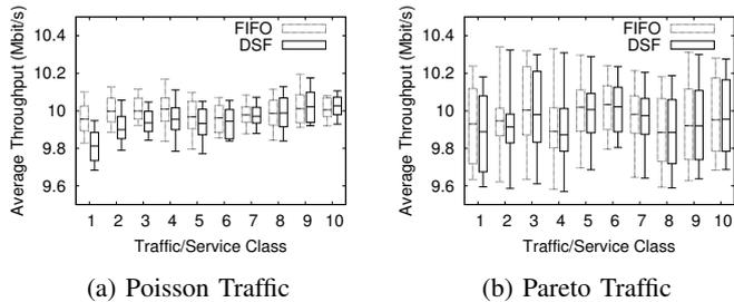
Fig. 7: Multiple Classes - FIFO vs. DSF
