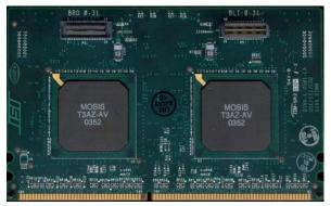
Figure 1. DIVA DIMM with two PIMs.
