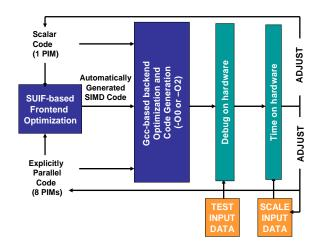
Figure 6. Performance Tuning Process on Hardware.
