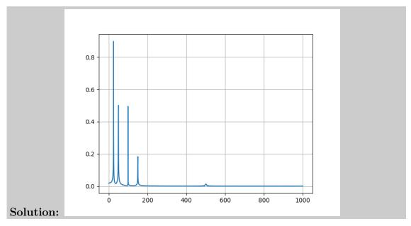
(b) Wavelet analysis: The DFT/FFT spectrum can not indicate the start-end of the high-frequency injection. It can only provide information about the overall fre-
