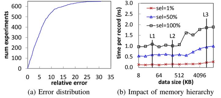
Fig. 3. Modeling single-threaded plans.
