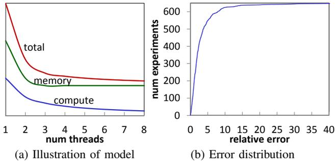
Fig. 4. Modeling multi-threaded plans.
