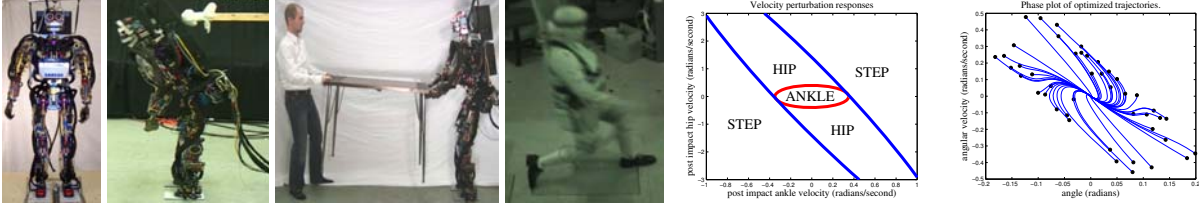
Figure 1: A: Our hydraulic humanoid robot standing on a moving platform used for clinical human balance testing. We compared the robot’s perturbation responses to human perturbation responses. B: The humanoid responding to a push (stick with white padding on end). C: The humanoid collaborating with a human to lift a table. D: Human slipping experiments. This video image was shot with infrared illumination, because the experiment is done in darkness to conceal the slipping location from the subject. The subject’s left foot has just slipped on a puddle of glycerin, and the right foot has come down from its swing and is pressing against the floor in an attempt to recover. E: An error response classifier for a simple optimal control model of standing balance. The axes are the ankle and hip velocities after an impulsive perturbation. For small perturbations, ankle torques are primarily used for the response. Larger perturbations in a particular direction are handled by recruiting hip muscles. Other large perturbations are handled by taking a step. F: A conceptual example of a continuous response generator based on storing trajectories. These are a set of optimized ankle responses to balance perturbations. The black dots are the initial state after the perturbation.
