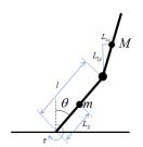
One Degree-of-Freedom sagittal model: A constrained 2-link inverted pendulum
