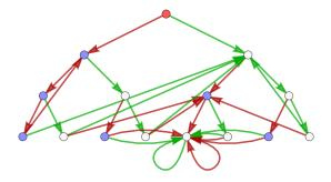
The frontier automaton for  $a^\star b^\star a$  at level 4. Back-edges go to the first possible place.
