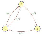
Each state p in C determines a transduction  $C(p): \mathbf{2}^* \to \mathbf{2}^*$  if we think of p as the initial state and all states as terminal (these devices are also known as output modules). For simplicity we simple write p for C(p).
