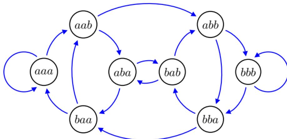
Here is the corresponding diagram, rendered in a particularly brilliant way. This is a so-called **de Bruijn graph** (binary, rank 3).
