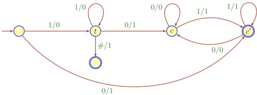
This version is obtained by a bit of surgery on the vanilla machine: handle 1:01, and split state  $c$  to eliminate trailing zeros.
