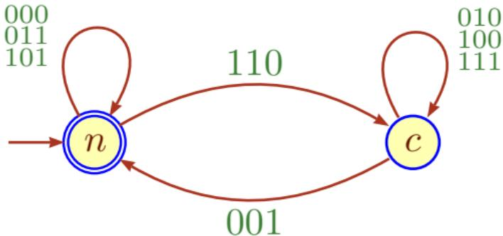
This is the logical core of any synchronous transducer for addition, a standard ripple carry adder.
