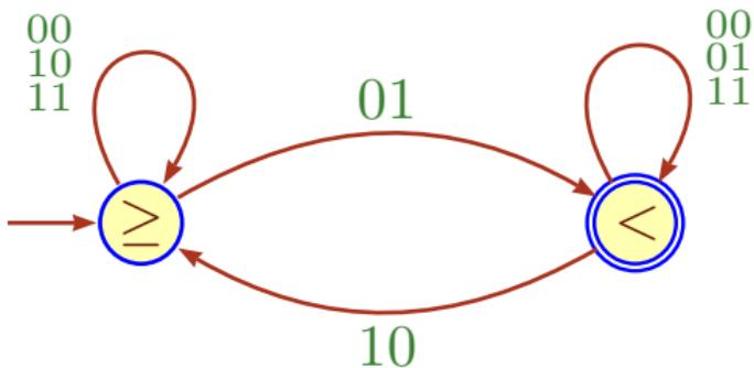
The basic comparison transducer: 0:1 leads to acceptance, 1:0 leads to rejection.
