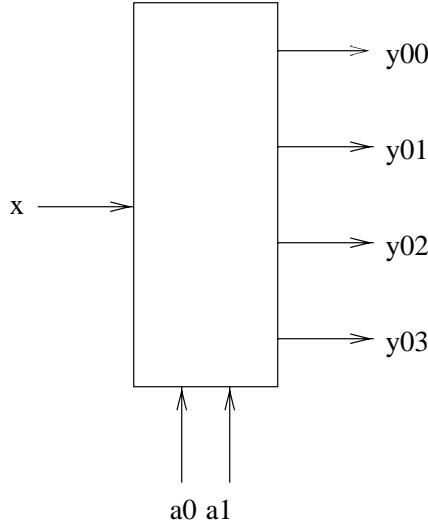
A demultiplexer works as follows. The value of  $x$  is transferred to the output line specified by  $a_0$  and  $a_1$ , i.e.,  $y_{a_0 a_1} = x$ . The value on all of the other outputs is 0. As an example, if  $x = 1$ , and  $a_0 a_1 = 01$ , then  $y_{01} = 1$  and  $y_{00} = y_{10} = y_{11} = 0$ . As another example, if  $x = 0$ , then independent of the value of  $a_0 a_1$ ,  $y_{00} = y_{01} = y_{10} = y_{11} = 0$ .
