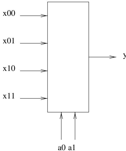
It has four data inputs,  $x_{00}, x_{01}, x_{10}, x_{11}$ , two control inputs  $a_0, a_1$ , and one output,  $y$ . The value of  $y$  is equal to the input specified by the binary number  $a_0a_1$ , i.e.,  $y = x_{a_0a_1}$ . As an example, if  $x_{00} = 1, x_{01} = 1, x_{10} = 0, x_{11} = 1$  and  $a_0a_1 = 10$ , then  $y = x_{10} = 0$ . A multiplexor is also called a *selector* because the control lines select from among the possible inputs.
