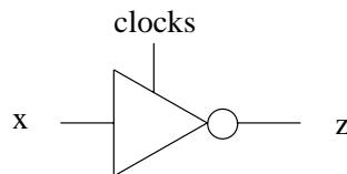
For our purposes, we can ignore the distinctions between the two clocks and view the two clock transitions as a single *pulse*. The input  $x$  can change anytime before the clock pulse arrives without affecting the value of  $z$ . When the pulse occurs, the value at  $x$  is sampled, and shortly thereafter,  $z$  takes on its new value (the opposite of the value that  $x$  had before the pulse occurred). Notice that a clocked NOT gate behaves differently from an unclocked
