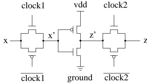
The clocked NOT gate actually uses two clocks, whose signals are interleaved as shown below. (Real processors typically have even more than two clock signals.)
