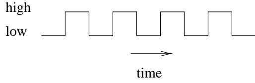
A clock is a periodic oscillating signal, as above. The high parts indicate a value of 1, and the low parts a value of 0. These days clocks are very fast, and can oscillate at speeds up to 1 Ghz (1 billion times per second)!
