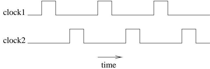
Here's how the clocked NOT gate works. When clock1 goes high, the value at  $x$  is carried over to  $x'$ . This causes the output  $z'$  to change (if necessary) to the new value,  $\overline{x'}$ . When clock2 goes high, the new value of  $z'$  is carried over to  $z$ .
