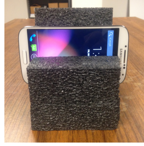
Fig. 7: Calibrating accelerometer along three axes. We collect measurements along all 6 directions ( \pm x, \pm y, \pm z ).
