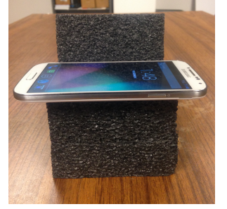
Fig. 7: Calibrating accelerometer along three axes. We collect measurements along all 6 directions ( \pm x, \pm y, \pm z ).
