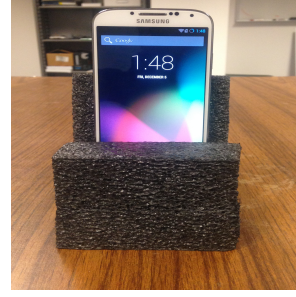
Fig. 7: Calibrating accelerometer along three axes. We collect measurements along all 6 directions ( \pm x, \pm y, \pm z ).
