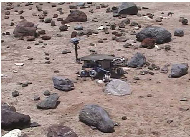
Figure 1. FIDO research rover prototype autonomously traverses rough terrain at Caltech Jet Propulsion Laboratory Mars Yard.
