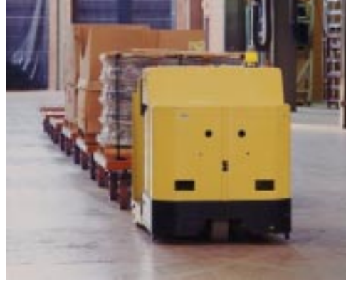
Figure 5: Tug AGV. This automated guided vehicle is one of three with mosaic positioning installed.
