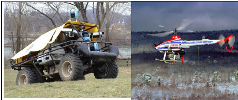
Fig 1: Autonomous Ground and Air Vehicles. A Honda ATV and Yamaha Rmax Helicopter were retrofitted for autonomy.
