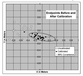
**Figure 4:** Residuals before and after calibration. The black squares are transformed into the white squares by systematic model calibration. The grey ellipse captures the remaining variance.
