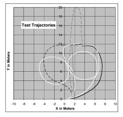
Figure 3: Calibration Test Trajectories. All start at the origin. All terminate near the point (3,12) with arbitrary heading..
