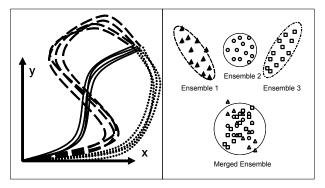
**Figure 1:** Visualization of Calibration Random Process Ensembles. Three ensemles are illustrated and only one of the trajectories in each is randomly selected. The reference trajectories of all ensembles must have one or more points in common to be used for calibration. This is only true of the endpoints in the figure.
