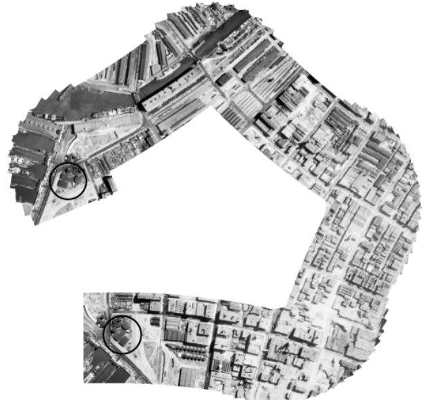
Figure 4: Mosaic constructed using only initial pose estimates from dead-reckoning. Note the discrepancy in alignment of the circled feature at the crossover point (lower left corner).
