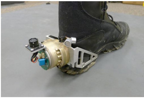
Figure 6. HG1930 IMU mounted on standard issue boot. Sonar transceivers (silver cylinders). Mil-spec connector runs cabling to backpack computing.
