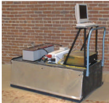
Figure 1: The mapping rig consists of a downward-looking camera system, to acquire the images, and an odometry positioning system, to determine a relative position of each image.
