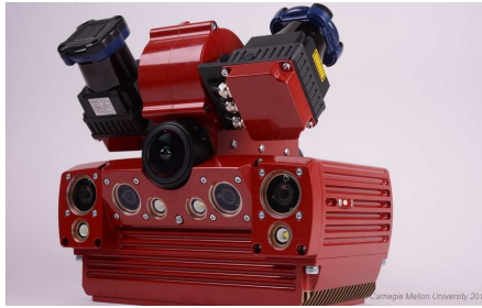
Fig. 2 A close-up of CHIMP's head, containing stereo cameras for visual odometry, amongst other sensors.
