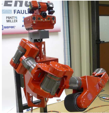
Fig. 8 A partially constructed CHIMP on a test-rig. The sensor head containing visual odometry sensors and a single arm are shown. The IMU is located in a temporary enclosure at the base of a mobile frame (not shown).
