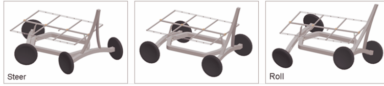
Fig. 3 Zoë's axles are free to rotate in both the steer and roll angles
