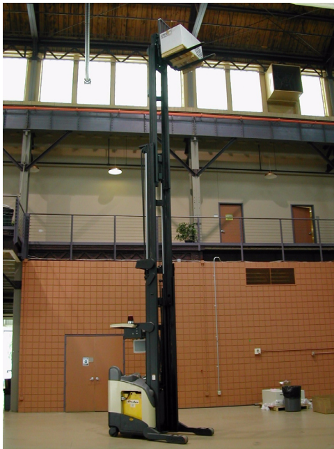
Figure 4: Vehicle test bed: mast extended to 340 inch high.
