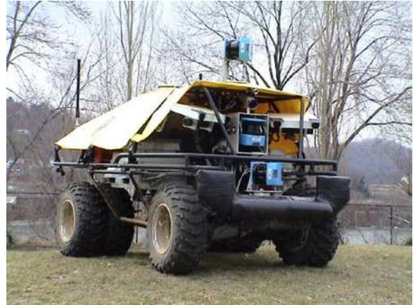
Figure 1: The PerceptOR off-road mobile robot. The experiments were performed with vehicles similar to the one pictured here.
