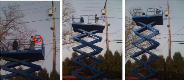
Fig. 4. We simulated a UAV flight using a hand-held mono-pod (red circle) and 15 meter platform lift.
