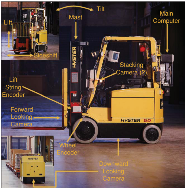
Figure 1. Vehicle retrofits. The tug AGV (bottom left) has a single downward-looking camera mounted to the chassis in the center of the vehicle. The fork truck (right) has two stacking cameras (cameras used for automated stacking) mounted to the roll bars and a forward-looking camera that moves with the forks. The lift and side-shift degrees of freedom of the mast are shown in the top left. A wheel encoder is attached to a small wheel that rides on top of the main drive wheel as shown. String encoders measure motions of the mast. LADARs that are normally mounted on the rear of the fork truck and the front of the tugger are not shown.
