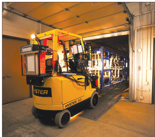
Figure 12. End unloading. The robot is removing the rack of auto parts from the trailer through the loading door. Note the lights of the visual guidance system under the robot.
