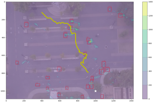
Fig. 3: Intermediate path plan with overlaid pedestrian trajectory prediction-based costmaps. The goal is at the white star (bottom right)
