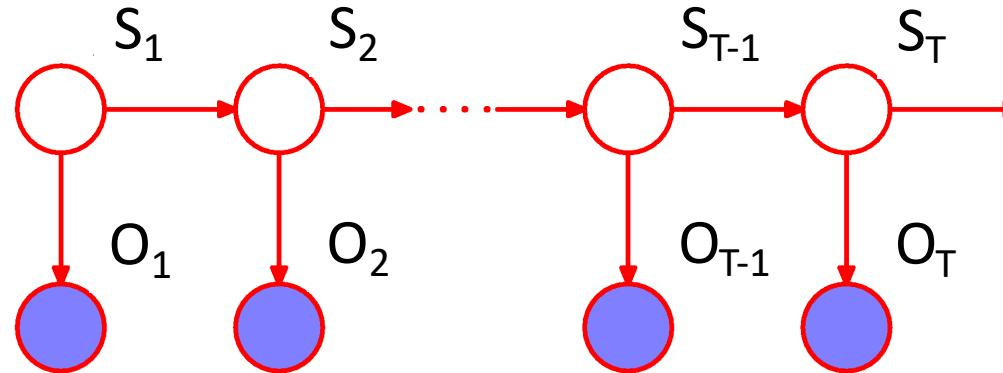
$$p(S_1, \dots, S_T, O_1, \dots, O_T) = \underbrace{\prod_{t=1}^T p(O_t | S_t)}_{\text{1st order Markov assumption}} \underbrace{\prod_{t=1}^T p(S_t | S_{t-1})}_{\text{can be extended to higher order}}$$
