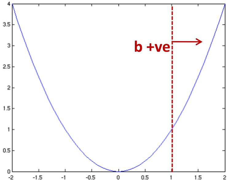
$$\begin{aligned} & \min_x x^2 \\ \text{s.t. } & x \geq b \end{aligned}$$
