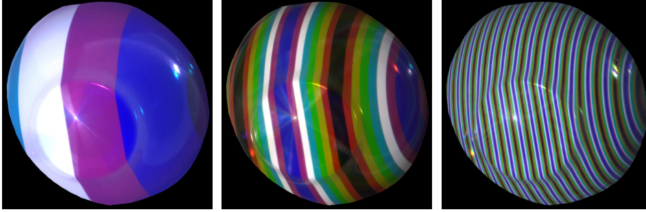
(d-f) Input images for concave bowl using color Gray codes
