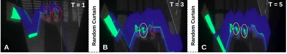
Figure 7.4: We illustrate the benefits of placing random curtains (that come with probabilistic guarantees of obstacle detection) while estimating safety envelopes, shown in SYNTHIA [ZBGGV + 19], a simulated urban driving environment. The blue surfaces are the estimated safety envelopes, and the green points show regions of high light curtain intensity (higher intensity corresponds to better estimation). There are three pedestrians in the scene. (a) Our forecasting model fails to locate two pedestrians (red circles). (b) The first random curtain leads to the discovery of one pedestrian (yellow). (c) The second random curtain helps discover the other pedestrian (second yellow circle). The safety envelope of all pedestrians has now been detected.
