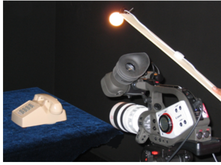
Figure 2.10: Setup: Our acquisition setup with a Canon XL2 video camera, a 60 watt light attached to a wand. In real experiments the camera and light source are further away to satisfy orthographic assumptions.
