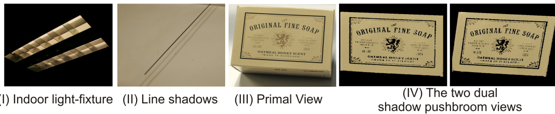
Figure 3.9: Line shadows from an indoor light fixtures: In (I) we show an image of a ceiling indoor light-fixture. The tubelights in the fixture act as line illuminants, producing a line-shadow (as in (II)). We use this to produce shadow pushbroom views of the scene shown in (IV).
