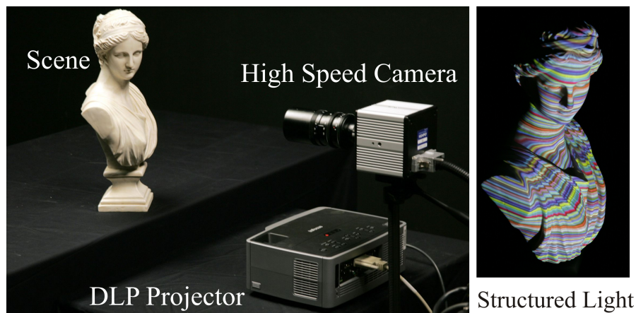
Figure 4.5: Illumination and acquisition setup for structured light based 3D reconstruction: The Photron high speed camera is placed vertically above the Infocus DLP projector. A vertical plane is placed behind the scene (statue) for calibration.
