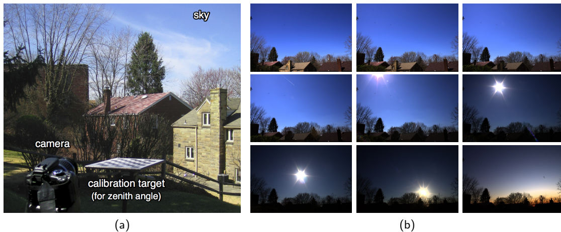
Figure 3.4: Ground truth data acquisition. (a) Acquisition setup. The calibration target, placed on a tripod in front of the camera and leveled with the ground, is used to recover the camera zenith angle. (b) Example images from 12:00 (top-left) to 20:00 (bottom-right), in one-hour increments. The images are shown with a linear camera response function.
