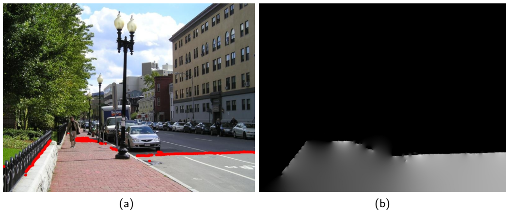
Figure 5.9: Estimating sunny regions on the ground. From our detected shadow boundaries (a), we generate a map of the ground region that is in sunlight by reintegrating the shadow boundaries only (b).
