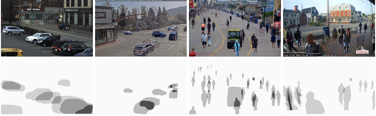
Figure 4.3: We illustrate generated training images(top) from Clip Art WALT dataset. The synthesized Ground-Truth amodal segmentation map(bottom) captures multiple layers(darker represents higher order of occlusion) of occlusions for training. The Clip Art images have realistic occlusions because the inpainting is performed by superimposing the object at the same location as it was observed but from varying time instances.
