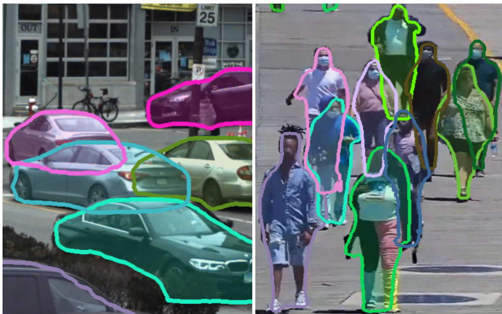
Figure 4.1: We visualize the prediction of amodal representation of vehicles and people under severe occlusions trained using our longitudinal self-supervision framework. The method shows significant improvement in amodal detection and segmentation with images captured from different cameras.
