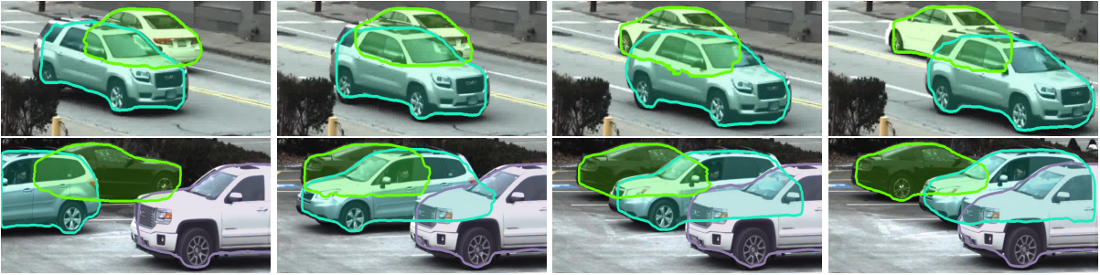
Figure 4.9: Accurate amodal segmentation of vehicles during occlusion while passing each other (Top) or when a vehicle is parking. Our method is able to provide consistent segmentation and detection of all the vehicles in severe occlusions and motions. This can lead to a drastic improvement in tracking objects with occlusions.
