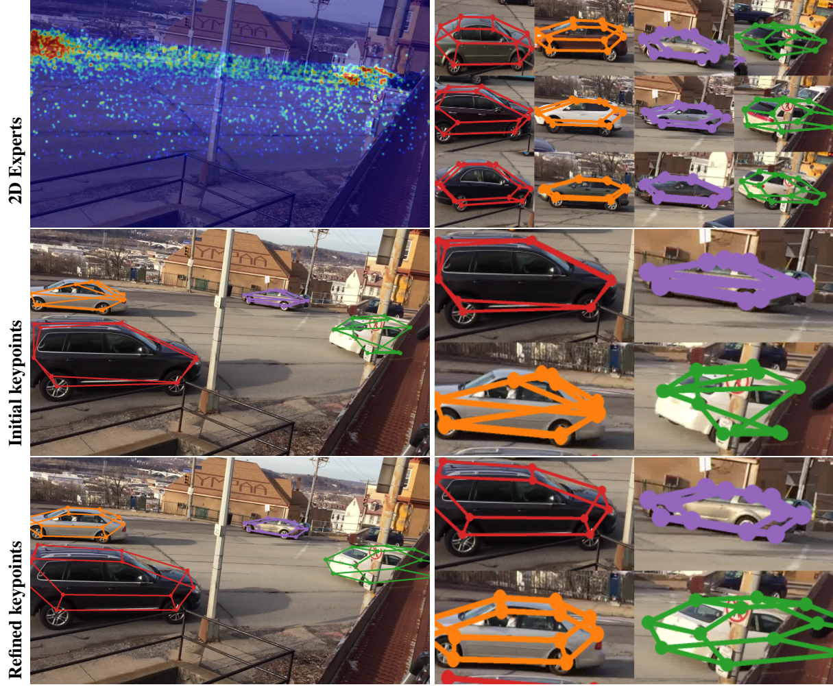
Figure 3.6: Examples of keypoint refinement via 2D longitudinal self-supervision. First row: Visualization of 2D experts. The heatmaps show frequency of 2D experts being used to refine other instances. 2D experts are used mostly at image border, occluded or far away places. The vehicle patches show the top three nearest neighbors retrieved from expert pool (good keypoints predicted by initial detector), which have very similar shape and pose to the refined instance; Second row: Initial erroneous keypoints from detector; Third row: Refined keypoints after 2D longitudinal self-supervision.
